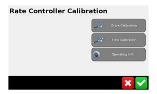
The 3<sup>rd</sup> option on this page is the <u>Operating Info</u> screen. Based on the information you have entered and calibrations you have carried out, this screen displays the basic operating parameters of your system.
