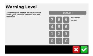
Enter an amount where you want a Low Tank <u>Warning Level</u> to appear on the screen. If an external Sonalert or Ez-Remote is connected, then this will also beep. The
