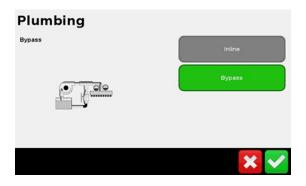
Inline - Where the Valve is "In-Line" with the Flow Meter and chokes the flow going to the boom. Commonly used on systems with Centrifugal Pumps, as Inline Valves can Deadhead the flow.
