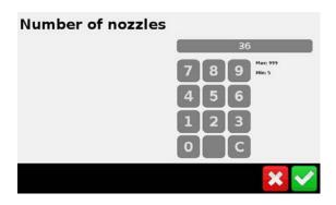
Enter the total <u>Number of Nozzles</u> on your boom. This includes extra nozzles fitted behind your wheels, etc. (make sure these are turned on as well). Press the Green Tick to return back to the <u>Rate Control</u> <u>Setup</u> screen.
