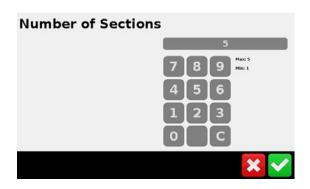
Enter how many Sections (Boom Valves) you are controlling. Press the Green tick.
