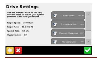
The <u>Drive Settings</u> screen will have the following options: <u>Target Speed</u>, <u>Proportional Gain</u>, <u>Minimum</u>
