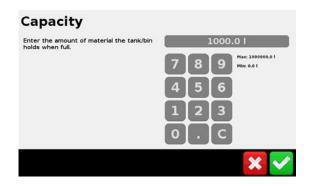
Enter your Tanks Capacity. If you fill it past its recommended capacity, then enter this full amount, as this affects the Low Tank level alarm, etc. Press the Green Tick when done. You will be returned back to the Tank/Bin Setup.
