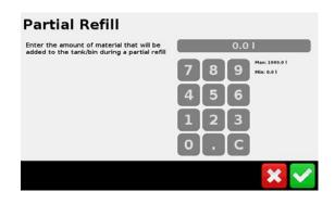
Enter the amount that will be added to the Tank if you are doing a <u>Partial Refill</u>. When this function is used, it will add this amount to the current volume in the tank. It will not just change the current volume to the amount entered here. If you are wanting to only refill a 4500L Tank to 3000L, then just adjust the Tank Capacity to 3000L.
