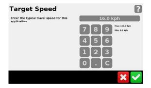
Enter the expected <u>Target Speed</u> you would be spraying at most of the time, then press the Green Tick when done. You will be returned back to the <u>Calibration Setup</u> screen.
