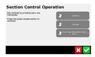
Latency - Use this to tell the controller how long it takes for Spray to come out after the command is given, as well as turning off again. (normally 0.5 to 2 secs)
