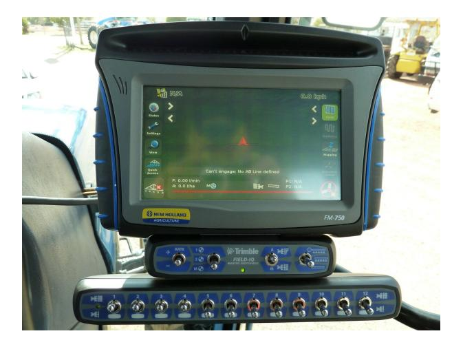
Setup, Calibration & Operation of Trimbles Field IQ Sprayer Control System, when used on the CFX-750 Display for Automatic Rate and Section Control.
