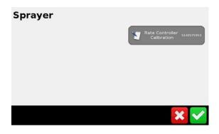
Verify that this is the correct serial number for the Module you are calibrating. Press the <u>Rate</u>
