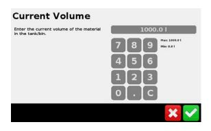
Enter the amount that is currnetly in the Tank, then press the Green Tick. You will be returned back to the **Tank/Bin Setup** screen.
