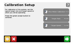
Verify the <u>Flow Meter Calibration</u> number is the same as the tag on your Flow Meter.
