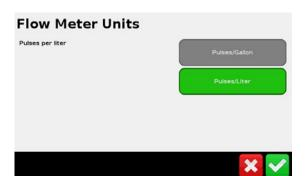
Select the applicable value for the reading on Flow Meter Calibration tag. Raven are normally Pulses per Gallon. Teejet, Midtech and Hardi are Pulses per Litre. Press the Green tick when done and you will be returned back to the **Feedback Setup** screen.
