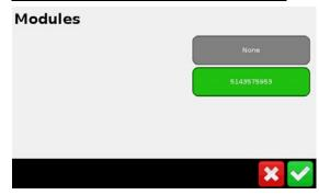
The Modules Screen will display. Any connected, or previously set-up modules will be displayed. Make sure you select the same serial number that is printed on your RSCM Module. Press the matching Icon.
