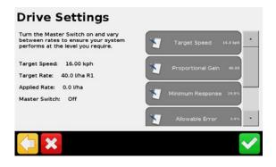
The right hand side of the screen displays current sprayer info, so you can operate while in this screen, to make these fine tuning adjustments. It is recommended to have a pressure gauge in your system, to observe for pressure oscilations while tuning. Press the Green Tick when done and you will be returned back to the **Rate Controller**Calibration screen.
