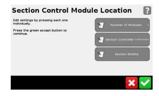
Verify that only 1 Module is selected and that the correct Serial Number is selected. **Select Section Widths**.
