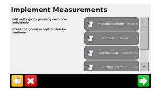
Always measure the width from the end nozzle, to the other end nozzle, then add one nozzle spacing to get the exact Implement Width.
