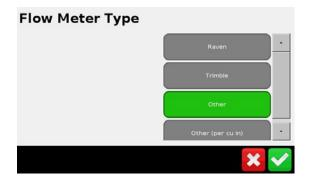
Select the brand of Flow Meter you have. (Use <u>Other</u> for Teejet), then press the Green Tick to return back to the <u>Feedback Setup</u> screen.
