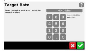
Enter the most common <u>Target Rate</u> you will be spraying at, then press the Green Tick.
