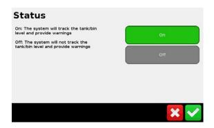
Select On to enable, then press the Green Tick and you will be returned back to the Tank/Bin Setup screen.
