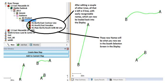
After loading the info back into the Display, it will come up as shown below, which will make it a lot easier to identify your correct AB Lines next time.
